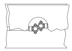
Optimize your rough configuration for a minimum C-C between hot & cold inlets (see examples). The orientation of the pair of supply connections is independent from the final spout position.
