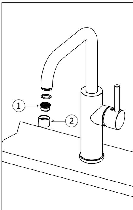
To clean the aerator (1), unscrew the aerator case (2) from the spout. Then pull out the aerator and soak in a vinegar and water solution to remove lime build-up. Once parts have been cleaned, reassemble by reversing steps.
